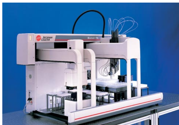
Figure 1. The Biomek FX liquid handler equipped with a 384-Channel Disposable Tip Head and a Span-8 Pipettor.
