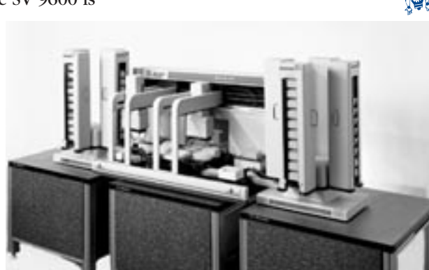
The Biomek FX automated system for the twelve-plate plasmid purification using the SV 9600 kit.
