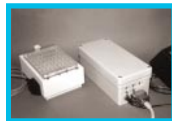
Figure 8: Magnet station, controller unit and power supply, above. Figure 9: Magnet station on the Biomek worksurface, below.
