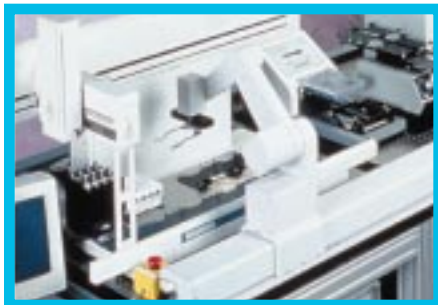
Figure 6. ORCA® arm moves 96-well plates from the Biomek® to the P/ACE System MDQ.
