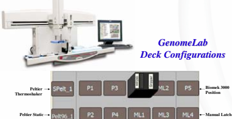
Figure 1. The Genomelab deck configuration is used for an automated method of purification of PCR products using the Biomek 3000 workstation. This configuration contains five positions for labware (P1-P5), four manual latch positions for tip boxes (ML1-ML4), a tool rack with gripper (Rack1), two dedicated positions for the Peltier Thermoshaker and Static devices and a disposal position for waste management. A customer provided thermocycler can be placed in position P5.
