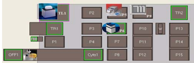
Fig. 2: BiomekFX workstation configuration: Tip Loader on TL1; Barcode reader on OFF1; Recirculating reservoir on P5; Orbital Shaker on P6; Reservoirs for solvents on P9 and Tip Trashes on TR1 and TR2
