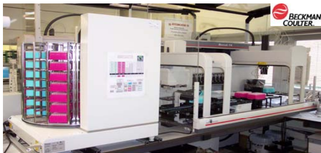
Fig. 1: BECKMAN-COULTER BiomekFX Dual-Arm LiHa with KENDRO Cytomat Carousel (capacity for 28 tip boxes and 70 DW plates)
