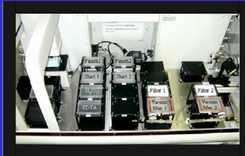
Figure 1: Biomek FX workstation set-up to run a two plate purification using the MultiScreen 384 -SEQ filters.
