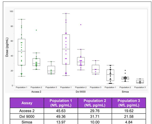
Figure 4. Endogenous NFL levels in EDTA plasma from three different groups with high, medium, and low levels of NFL on Access 2 (green dots), Dxl 9000 (purple dots), and Simoa (black dots). Table below shows median doses of NFL in each population group compared across the three different analyzers.
