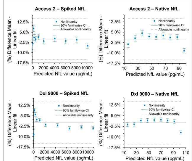
Figure 3. Linearity study was performed using K2 EDTA samples on the Access 2 and Dxl 9000 Immunoassay Analyzers. % Non-linearity was <10% across all concentrations evaluated, and for both spiked and native samples.
