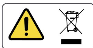
Customers must understand and follow all laws regarding the correct decontamination and safe disposal of electrical equipment. For Beckman Coulter products bearing this label, contact your dealer or local Beckman Coulter office for details on the take-back program that facilitates the correct collection, treatment, recovery, recycling and safe disposal of these products.
