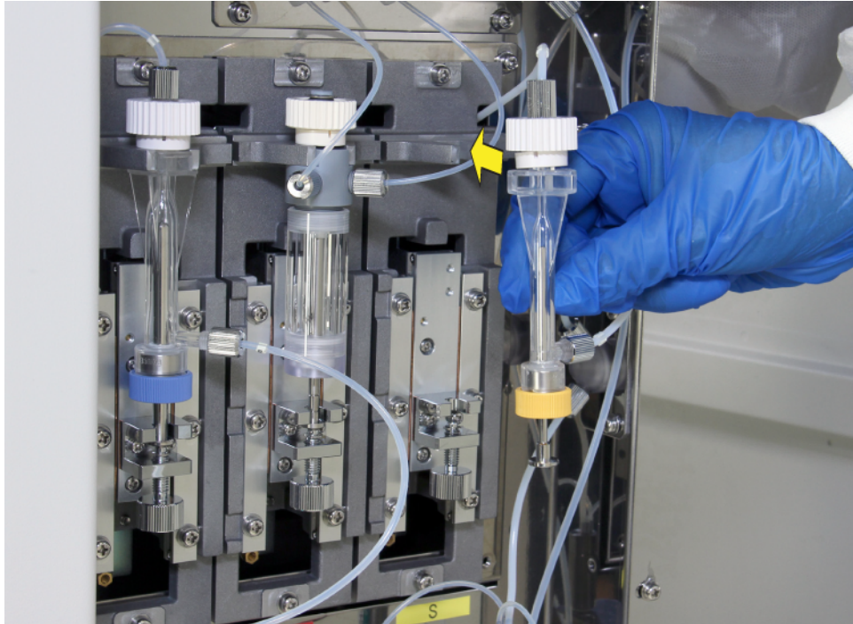
Figure 197 Installing the Sample Syringe Into the Mounting Groove
