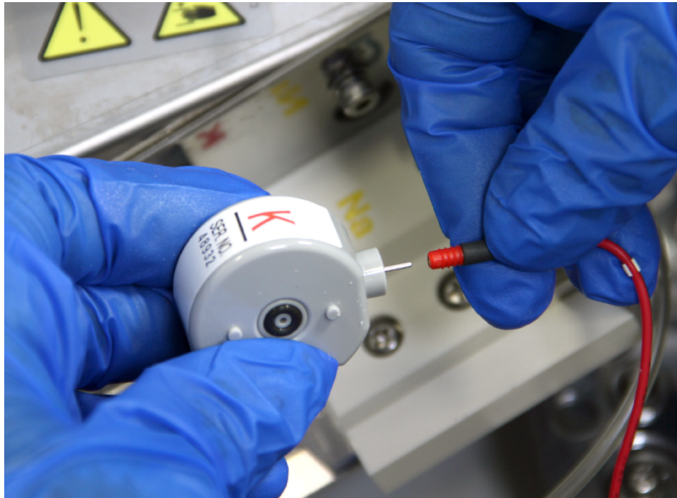
Figure 228 Connecting the Red Lead Wire to the K Electrode
