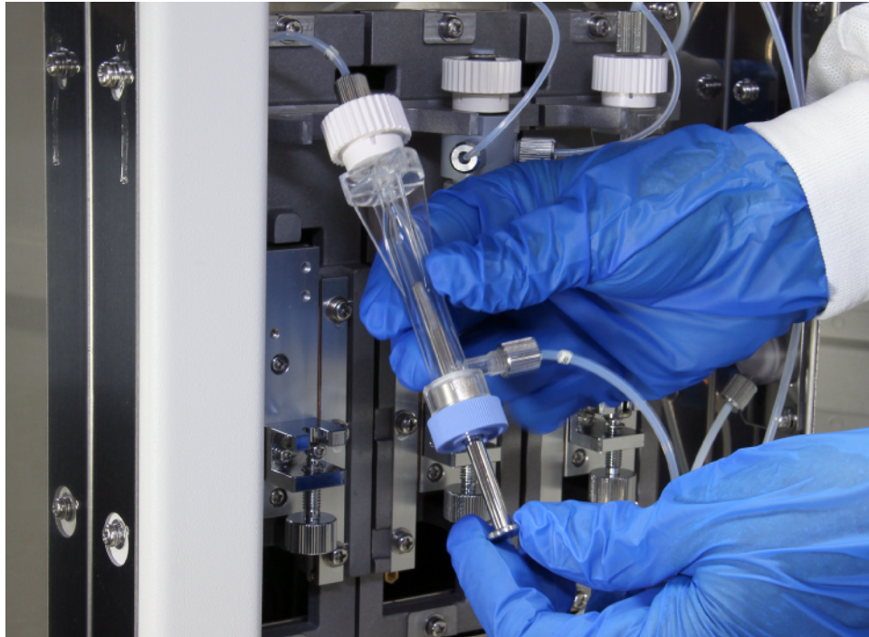
Figure 192 Moving the Syringe Piston Up and Down
