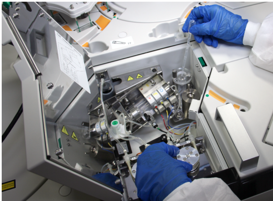
Figure 233 Pipetting ISE MID Standard Solution Into the Sample Pot
