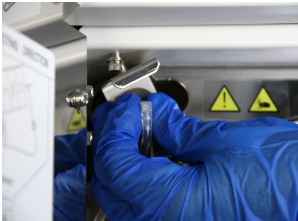
Figure 130 Putting the Drain Tubing on the Hook
