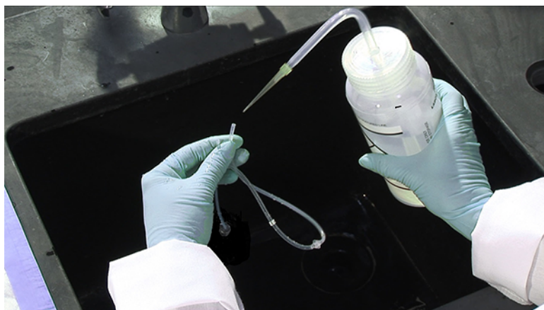
Figure 209 Sample Pot Tubing and Bypass Tubing
