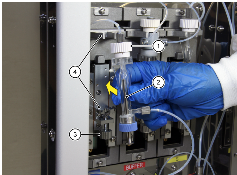
Figure 191 Installing the Syringe
