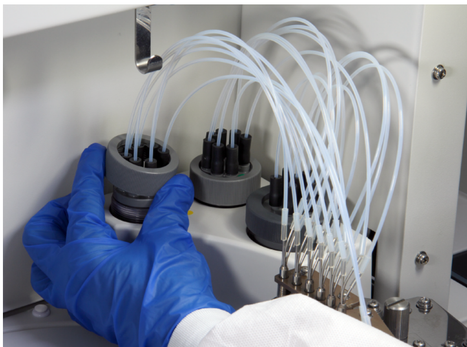
Figure 117 Returning Manifolds to Original Positions
