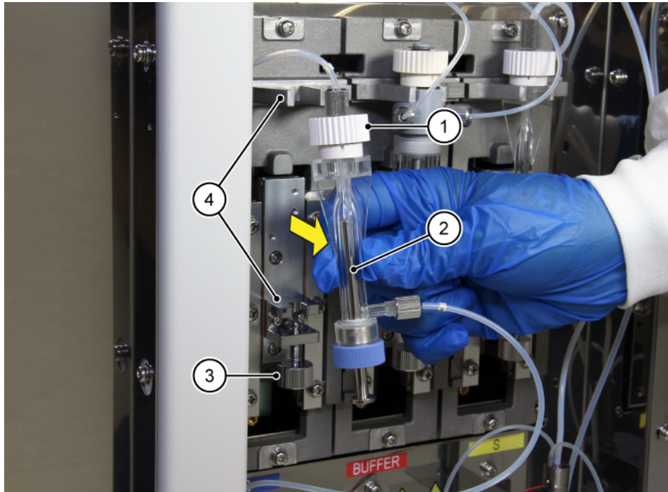
Figure 189 Remove the Syringe
