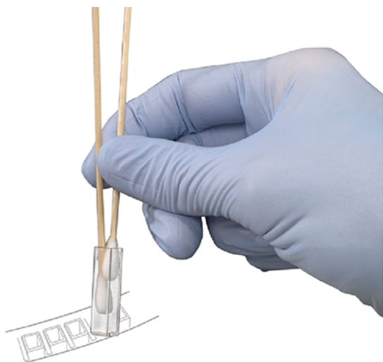
Figure 175 Removing the Cuvette
