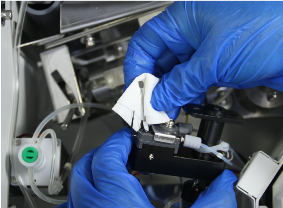
Figure 103 Wiping the Nozzles, the Liquid Level Sensors, and the Mix Bar
