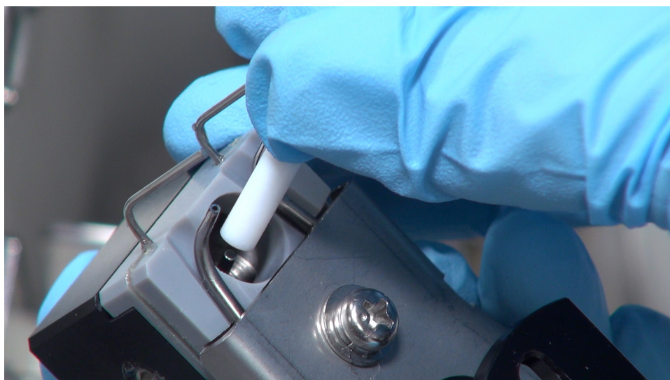
Figure 242 Inserting the New Mix Bar into the Shaft on the Mixing Subsystem
