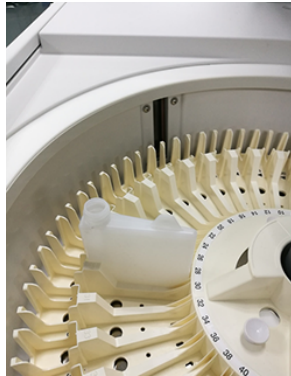
Figure 52 Placing 60-ml Bottle in Inner Ring
