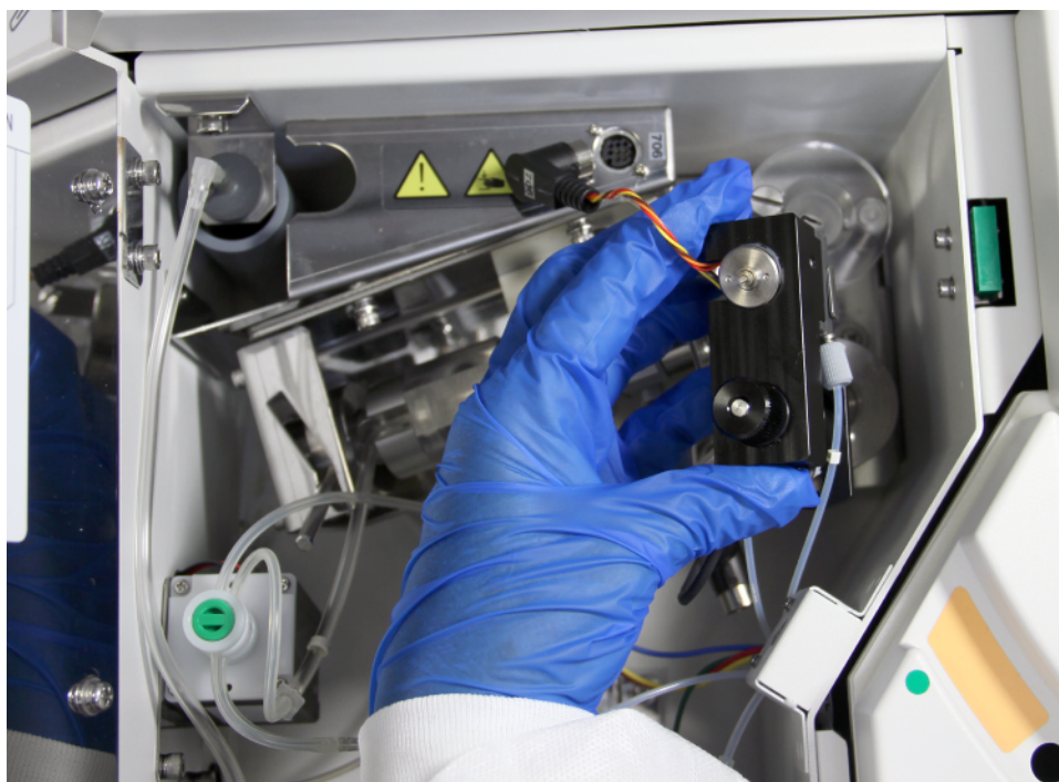
Figure 234 Putting the Mixing Subsystem Back Into Position
