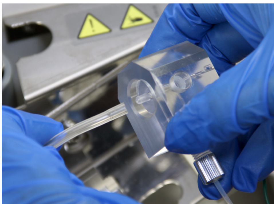
Figure 217 Attaching the ISE REF Electrode Block-side Drain Tubing (Labeled 6) and the ISE Reference Solution Tubing
