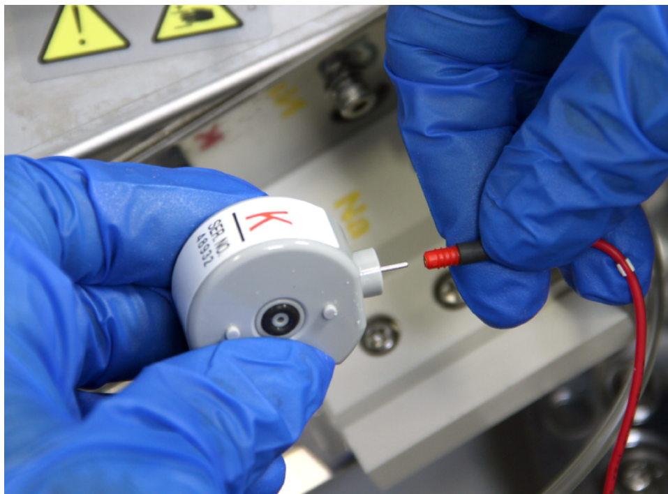
Figure 156 Connecting the Red Wire to the Electrodes
