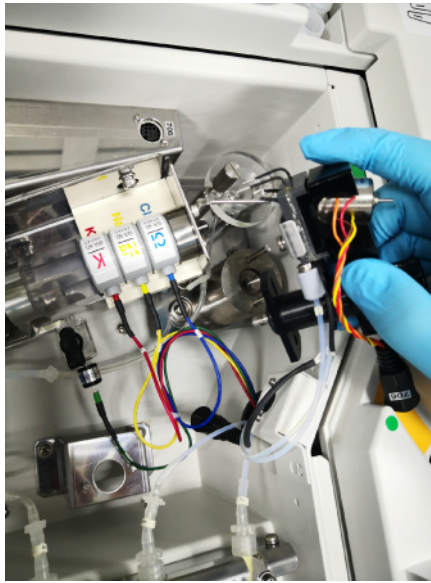
Figure 244 Unseating the Mixing Subsystem
