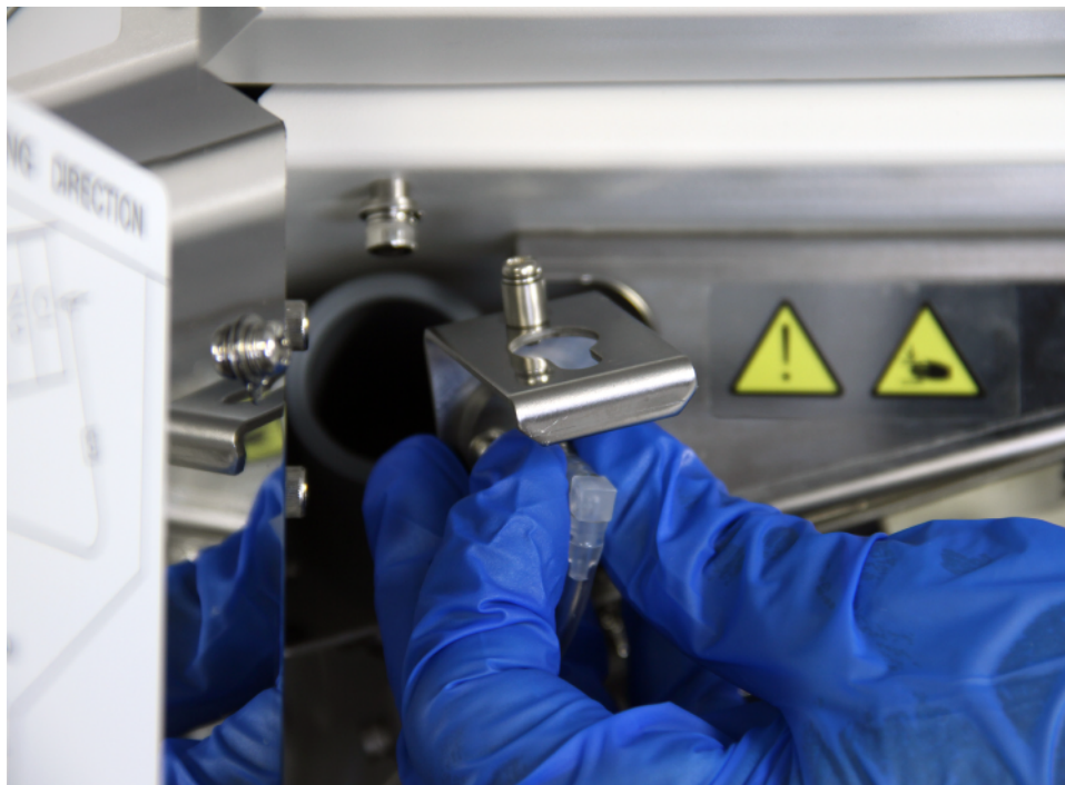
Figure 128 Removing the Drain Tubing
