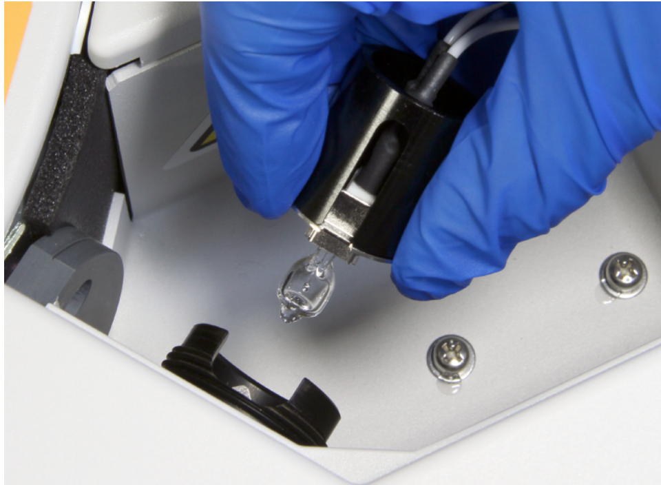
Figure 206 Aligning the Notched Collar of the Photometer Lamp
