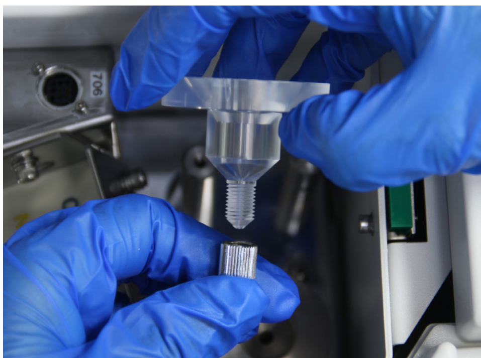
Figure 105 Unscrew the Connector
