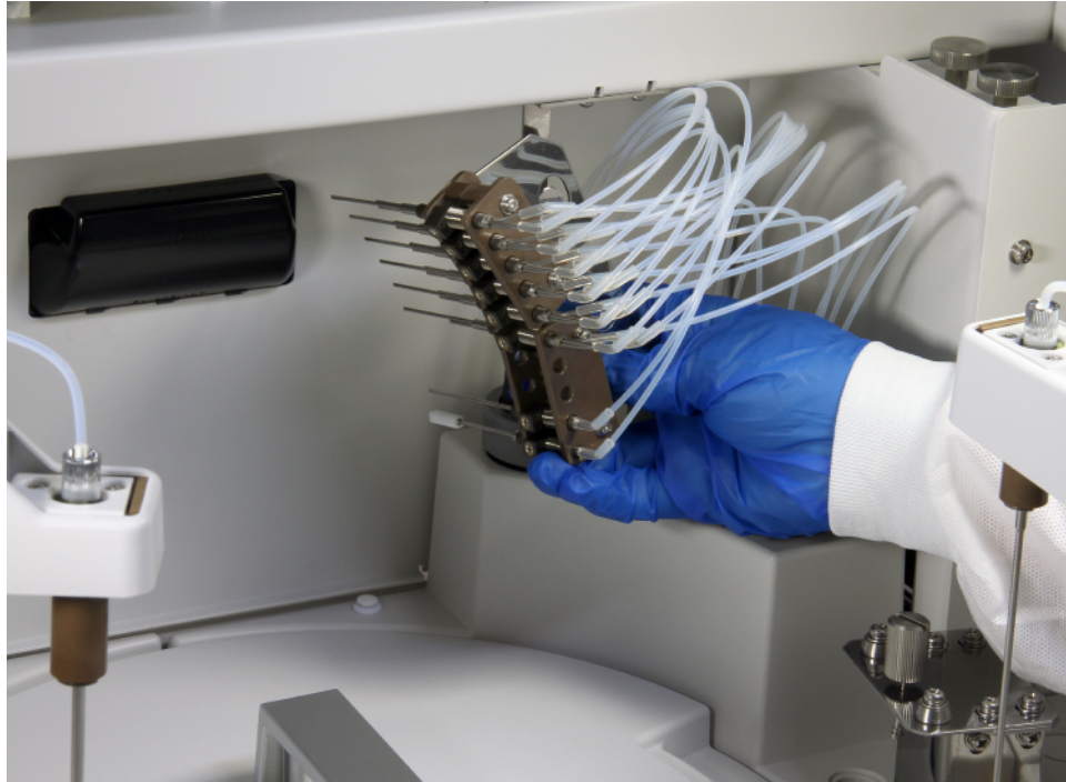
Figure 173 Removing the Wash Nozzle Subsystem
