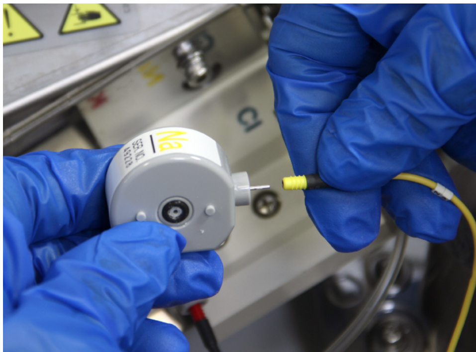
Figure 153 Connecting the Yellow Wire to the Electrodes
