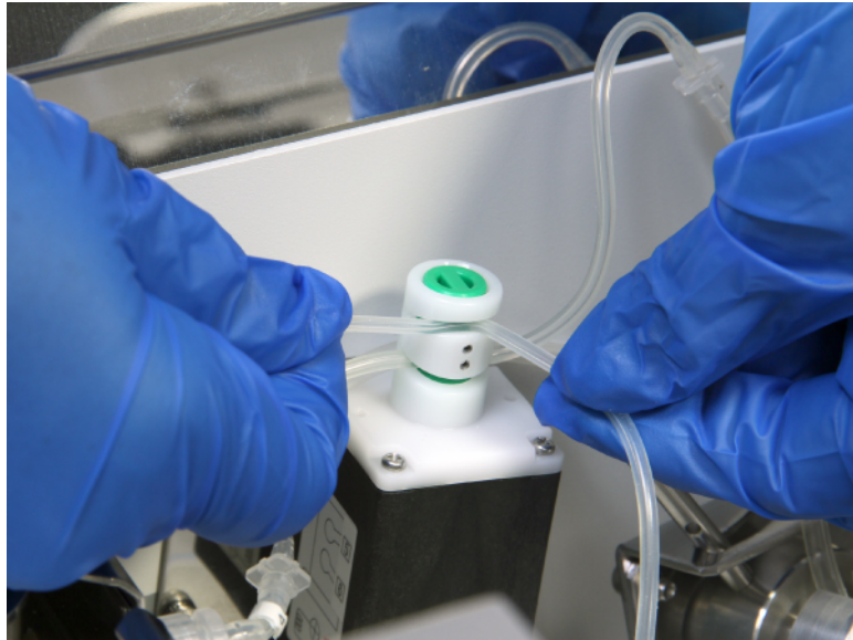
Figure 230 Removing the Tubing (Labeled 5 and 6) From the Pinch Valve
