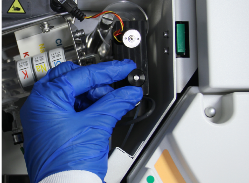
Figure 246 Reinstalling the Mixing Subsystem
