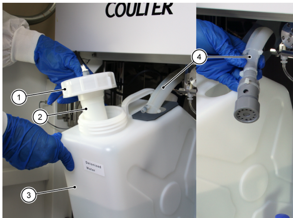
Figure 119 Float Sensor and Water Supply Tubing
