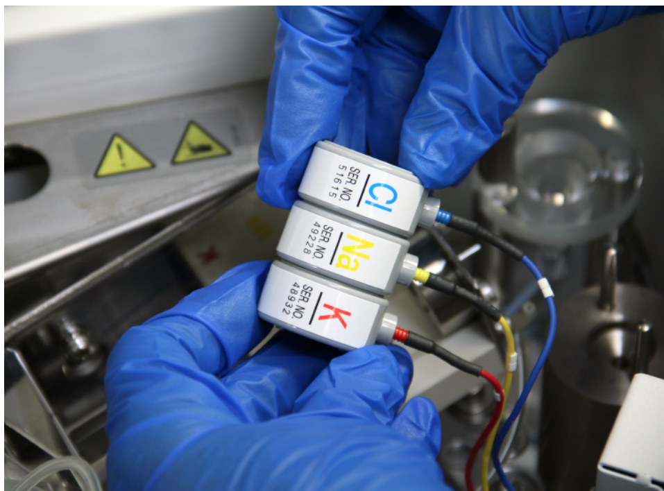
Figure 211 Removing the Electrodes from the Electrode Block
