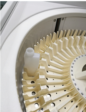
Figure 50 Placing 30-ml Bottle in Outer Ring
