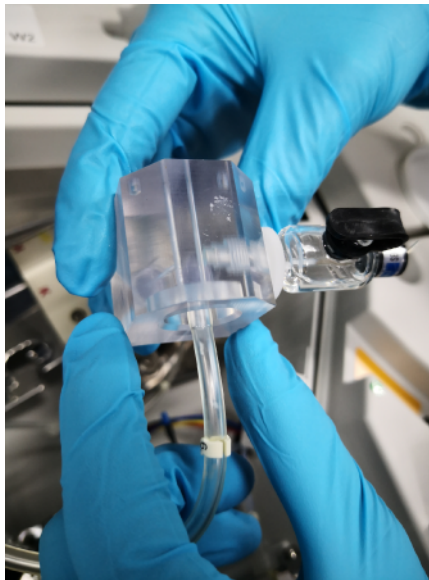
Figure 212 Removing the Electrode along with the Cap Screw
