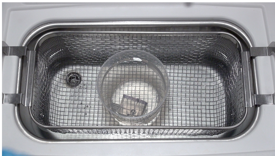
Figure 214 Sonicating the ISE REF Electrode Block
