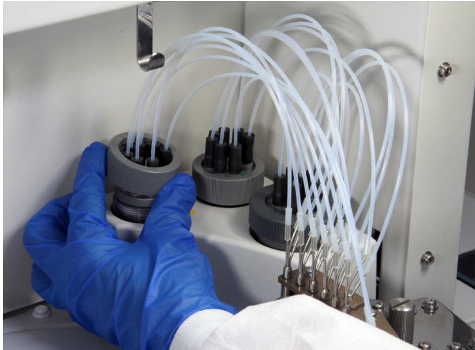
Figure 150 Returning Manifolds to Original Positions
