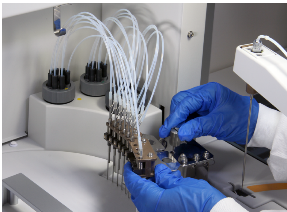
Figure 179 Putting the Wash Nozzle Subsystem Back in its Original Position
