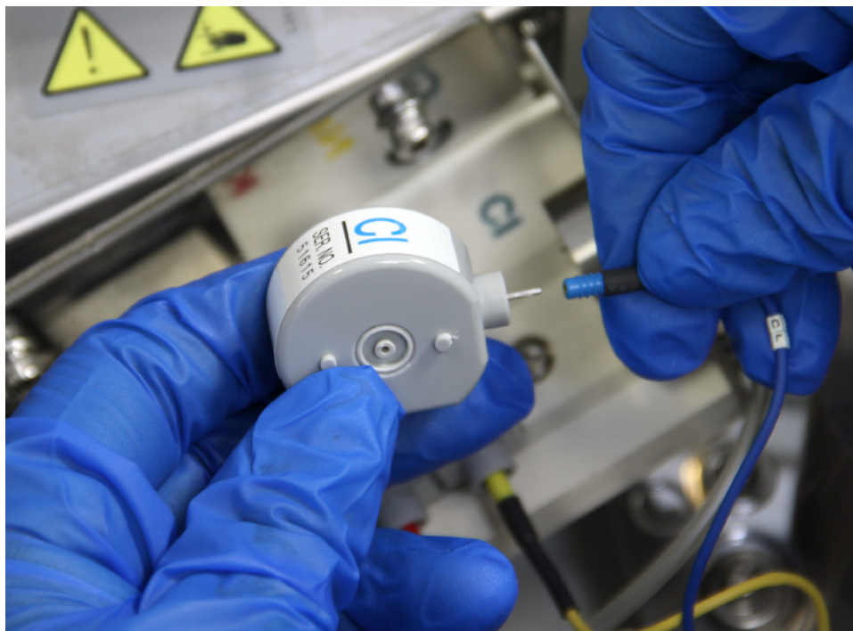
Figure 159 Connecting the Blue Wire to the Electrodes
