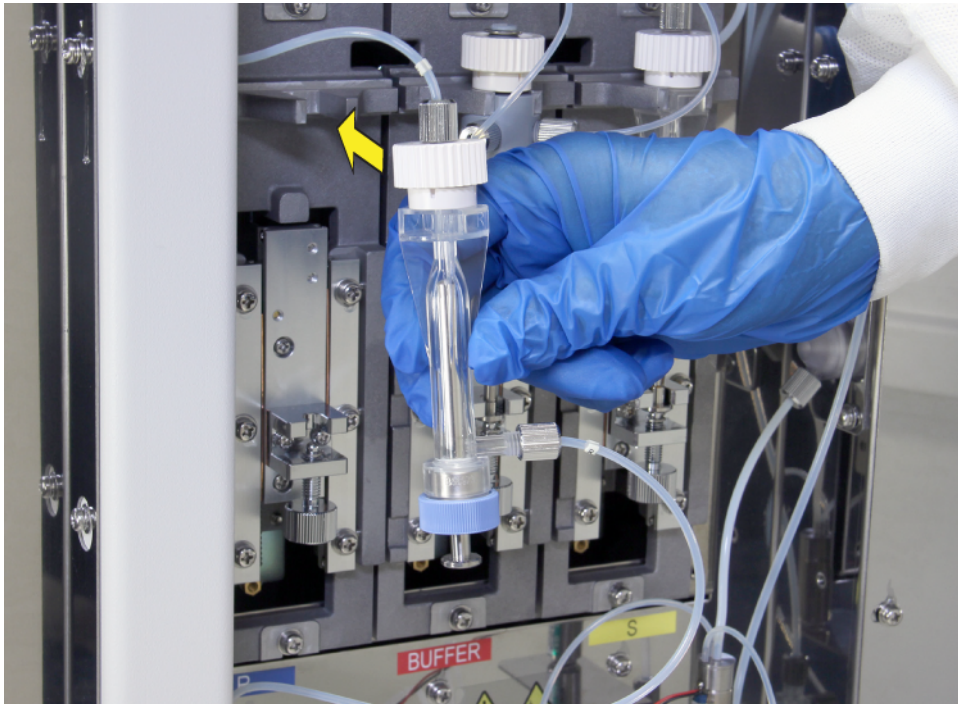
Figure 190 Installing the Reagent Syringe Into the Mounting Groove
