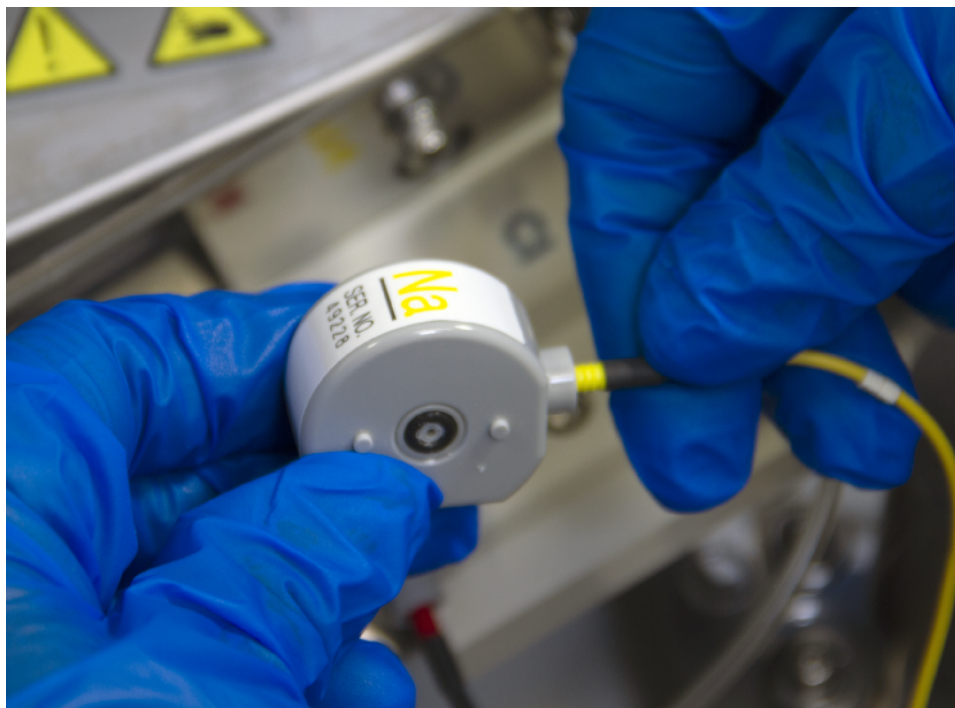
Figure 152 Disconnecting the Lead Wire of the Na Electrode
