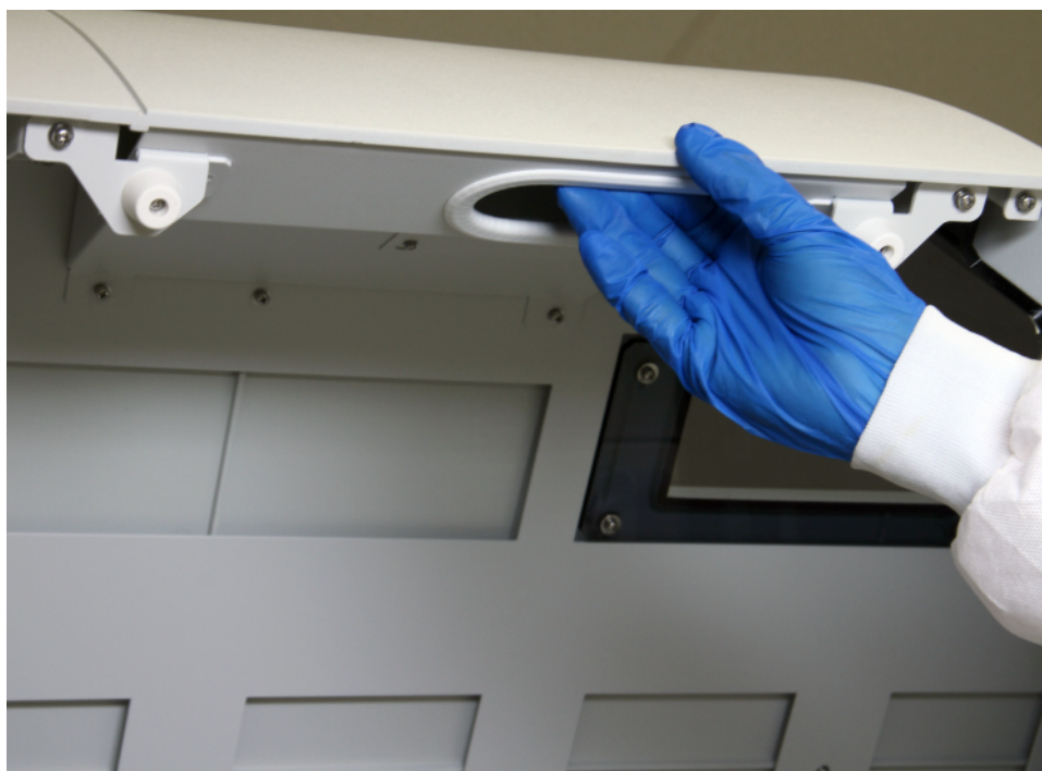
Figure 56 Correct Way to Grasp Analyzer Cover While Opening and Closing
