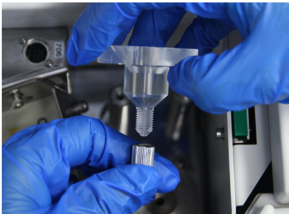
Figure 245 Disconnecting the Sample Pot Tubing From the Sample Pot
