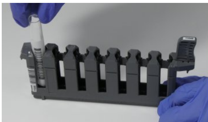
Figure 59 Placing a Sample Container in a Rack
