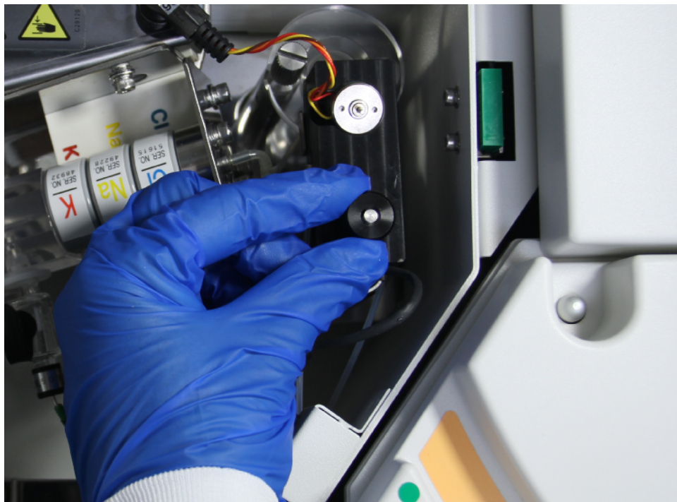
Figure 106 Reinstalling the Mixing Subsystem
