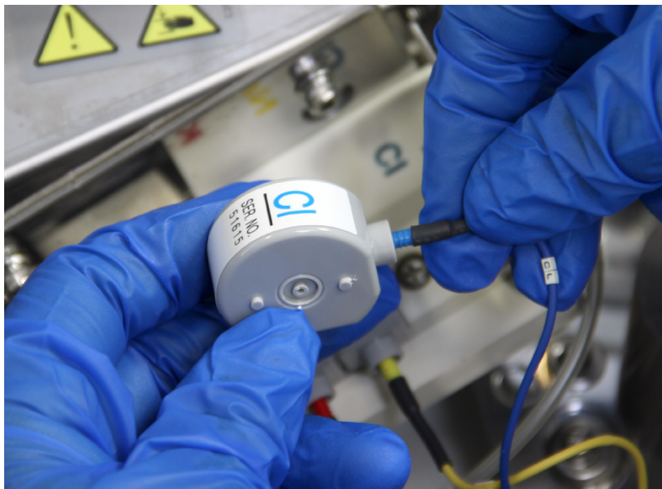
Figure 158 Disconnecting the Lead Wire of the Cl Electrode
