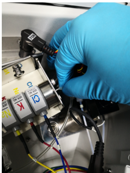
Figure 221 Removing the Sample Pot Tubing From the Electrode Block Inlet
