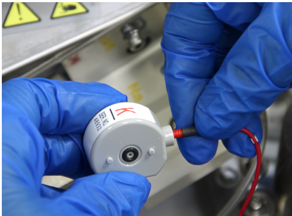
Figure 155 Disconnecting the Lead Wire of the K Electrode
