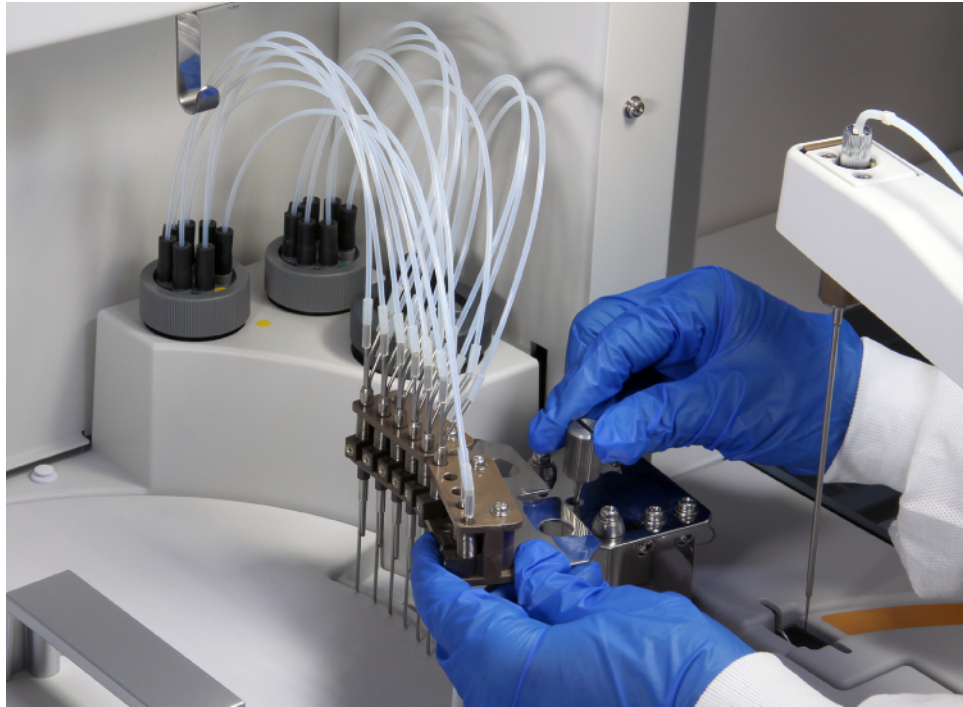
Figure 116 Returning the Wash Nozzle Subsystem to Original Position
