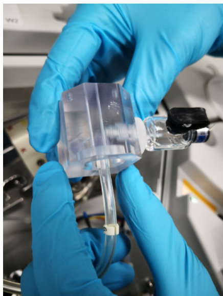
Figure 161 Removing the ISE REF Electrode
