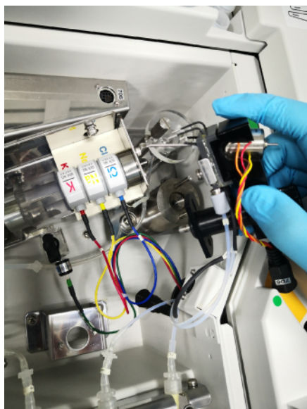
Figure 229 Unseating the Mixing Subsystem
