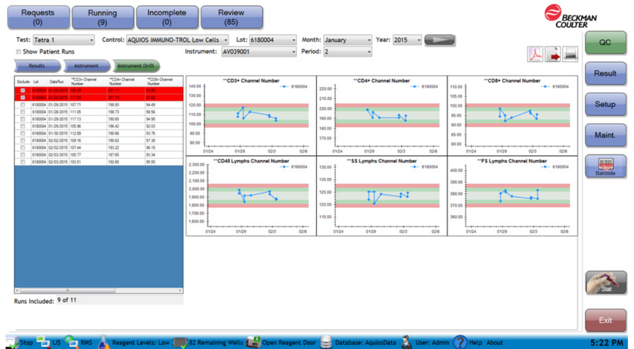
Figure 3.16 Instrument Drift Tab: AQUIOS IMMUNO-TROL Low Cells, Tetra-1
