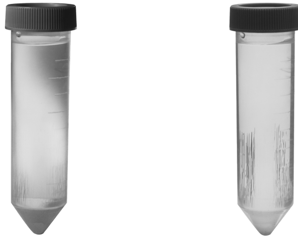
Figure 8. Examples of Tubes with Minimum and Moderate Crazing
