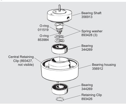
Figure 5.3 Exploded View of the Bearing Assembly
