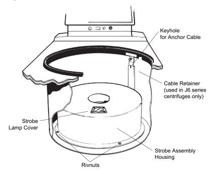
Figure 2.2 Installing the Strobe Assembly (J6-MI Centrifuges)
