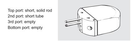
**9** Move the second chamber into place on the assembly opposite the first chamber.
