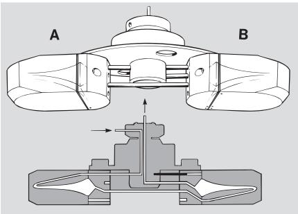
Figure 2.13 Chamber Assembly and Configuration for a Two-Chamber Run
