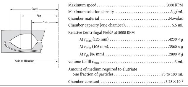
a. Relative Centrifugal Field (RCF) is the ratio of the centrifugal acceleration at a specified radius and speed ( $rw^2$ ) to the standard acceleration of gravity (g) according to the following formula: RCF =  $r\omega 2/g$  — where r is the radius in millimeters,  $\omega$  is the angular velocity in radians per second (2  $\pi$  RPM /60), and g is the standard acceleration of gravity (9807 mm/s<sup>2</sup>). After substitution: RCF = 1.12r (RPM/1000)<sup>2</sup>
