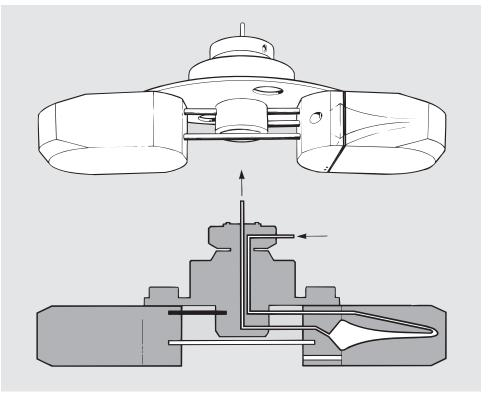
Figure 2.12 Chamber Assembly and Configuration for a Single-Chamber Run
