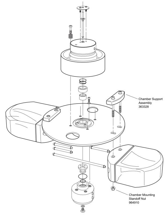
Figure 5.1 Exploded View of the JE-5.0 Quick-Release Assembly
