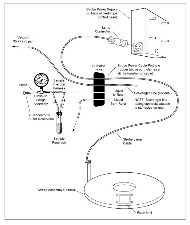
Figure 2.4 Electrical and Liquid Line Connections in Avanti J-26S XP Series and J-26 XP Series Centrifuges
