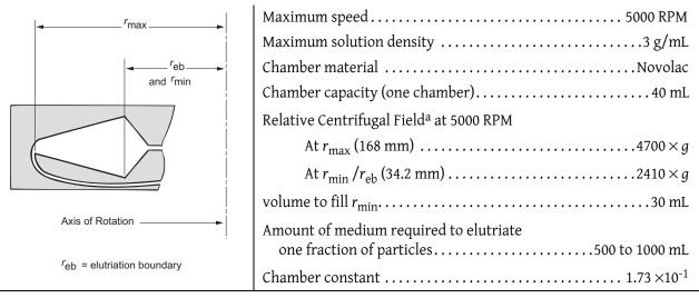
a. Relative Centrifugal Field (RCF) is the ratio of the centrifugal acceleration at a specified radius and speed ( $rw^2$ ) to the standard acceleration of gravity (g) according to the following formula: RCF =  $r\omega 2/g$  — where r is the radius in millimeters,  $\omega$  is the angular velocity in radians per second (2  $\pi$  RPM /60), and g is the standard acceleration of gravity (9807 mm/s<sup>2</sup>). After substitution: RCF = 1.12r (RPM/1000)<sup>2</sup>
