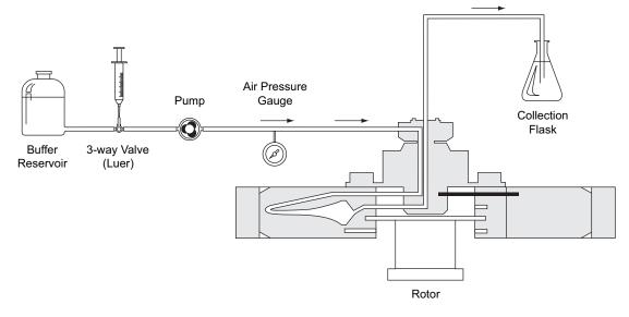
**2** Load sample into the syringe; attach the syringe to the injection valve.
