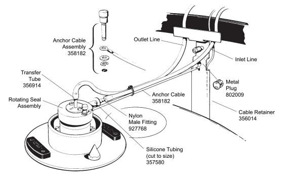
Figure 2.14 Attaching Tubing to the Seal Assembly (J6-MI Centrifuge Shown)
