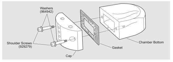
Figure 2.10 Elutriation Chamber Components
