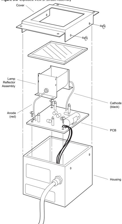
Figure 5.6 Exploded View of Strobe Assembly
