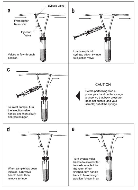
**2** Load the sample into a syringe with a luer fitting.
