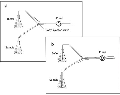
**2** When most of the sample has been drawn past the three-way valve, turn the valve back to the position shown in Figure 4.4b.
